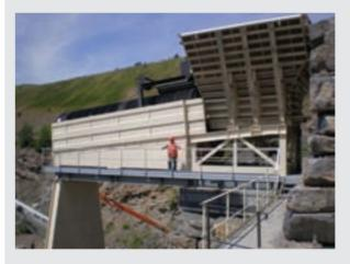
The reciprocating feeder is powered by a single hydraulic cylinder with both drive units supplied by independent hydraulic pumps coupled to electric motors. With the screen apertures being relatively small for this separation Holborne supplied and installed their patented barrel cleaner mechanism
