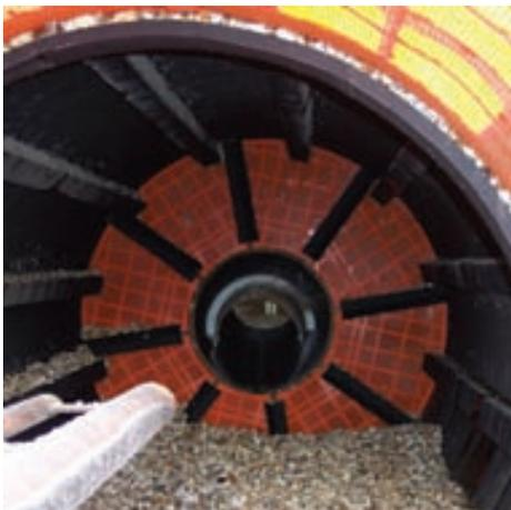
In essence, a barrel is incorporated within a processing plant when adhering clay or fines need to be liberated from the aggregate to produce a clean product.
