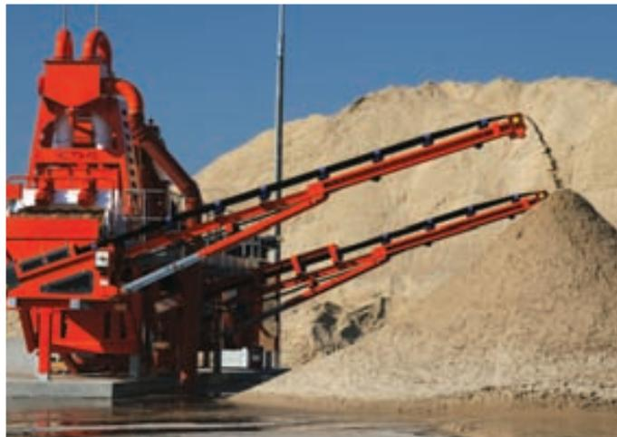
Once material has been delivered to the M2500 E4X the feed conveyor delivers the material to a double deck ProGrade P275 rinsing screen fitted with wire mesh on both decks. The +22m material is removed by the top deck and the 15-22mm by the bottom deck and these products are stockpiled by the integrated 9m wing conveyors.
