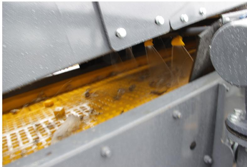
The top deck of this screen separates at +32mm and this material is sent to stockpile via one of the integrated wing conveyors. The bottom deck separates at 4-32mm and this material is then sent to the AggMax for scrubbing via the integrated Rotomax RX80 logwasher.
