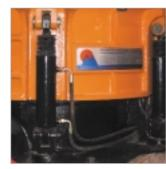
The hydraulic system is able to clear the crushing chamber of obstructions whilst returning the crusher to its pre-set dis-charge settings.
