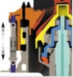
Schematic showing transducer returning upperframe to original position.
