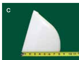
With elevator bucket back laid flat, measure the back depth
