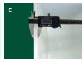
Using a caliper, measure the thickness of the bucket
