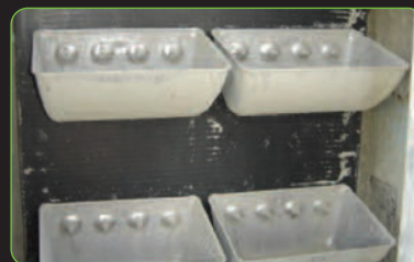
Starco Jumbo (SJ) Buckets on 4B Steel Web Core Belt in Cement Application
