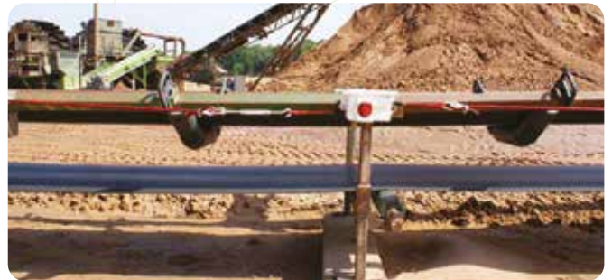
Pullswitch installed on open belt conveyor
