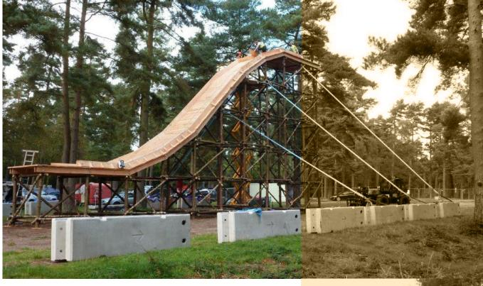
A clay model of a Rover 75, the last car produced at the Longbridge works nearby, was lifted onto the 10 metre high ramp by crane. Then the 1.5 ton car was made to freefall down the ramp and crash into the TVCB concrete safety barriers at the end of the safety zone.
