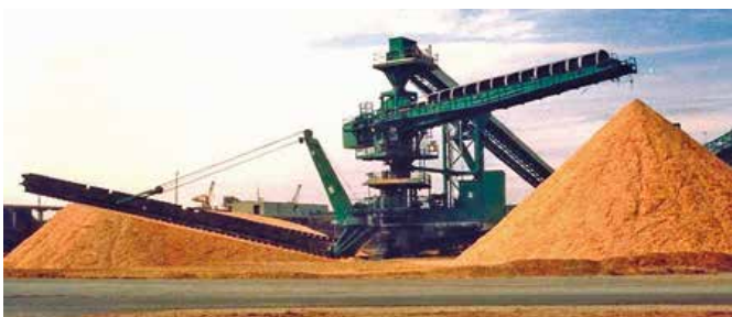
Circular Storage with Cantilever Reclaimer by SCHADE
