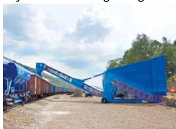
Stormmajor® Boom Feeder a flexible solution for Rail Wagon Loading
