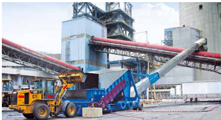
Stormmajor® Boom Feeder introducing fuels to an existing conveyor belt at Hong Kong Electric
