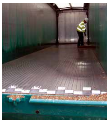
Self Discharging Walking Floor High-Cube Trailer
