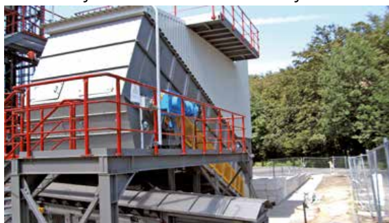
Weigh Belt Feeder gives Close Output Control
