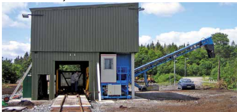
Discharge Direct from Samson® Box Feeder to Mobile Conveyor
