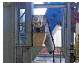
Discharge from Samson® Material Feeder to Vertical Bucket Elevator
