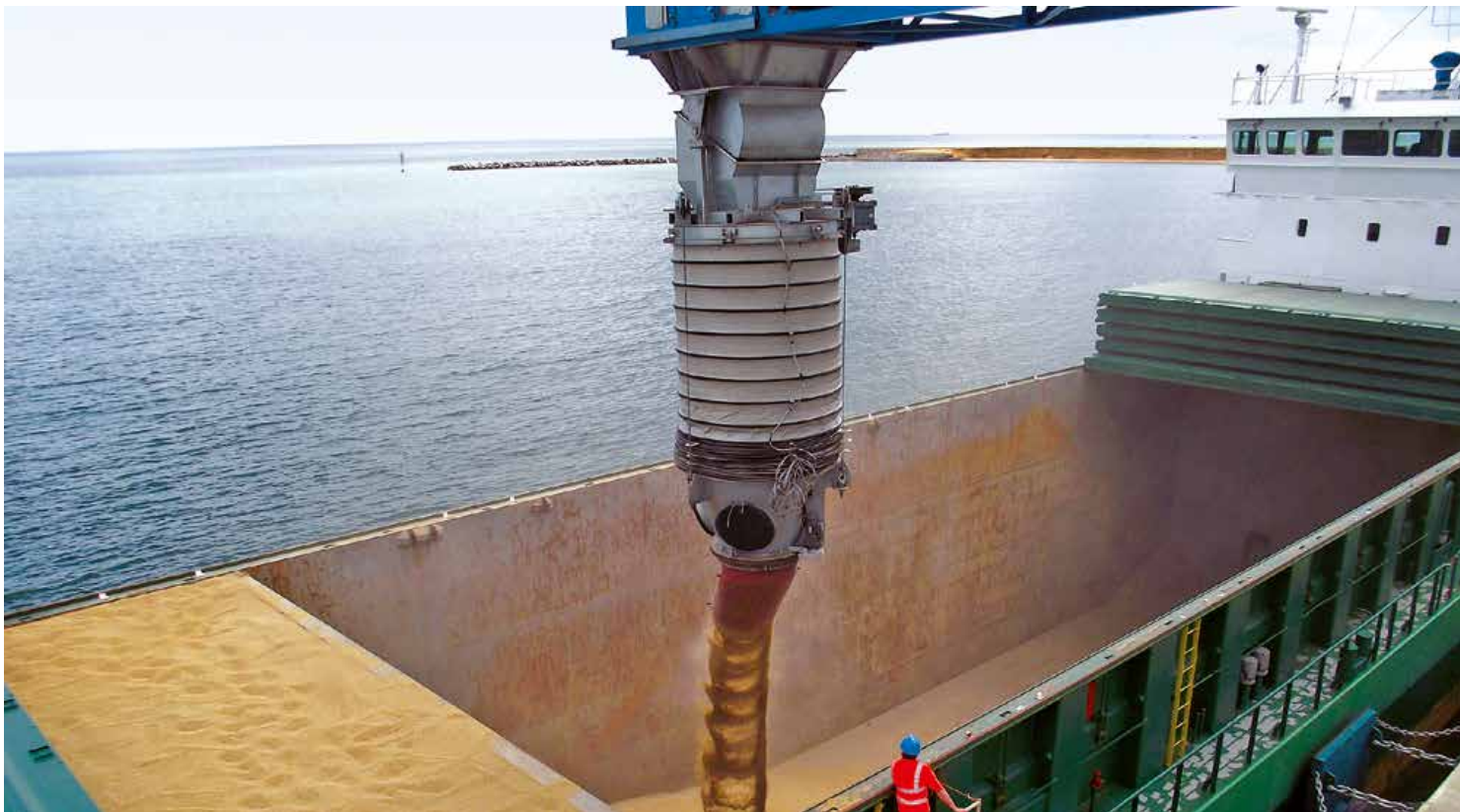
Rotating Trilling Chute for accurate material placement
