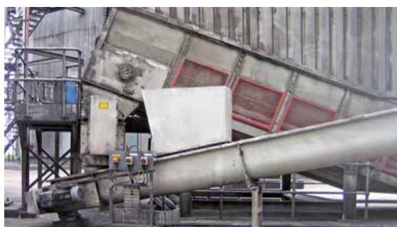
Transfer by Screw Feeder and Conveyor
