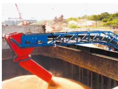
Twin Samson® Material Feeders mounted to the Shiploader
