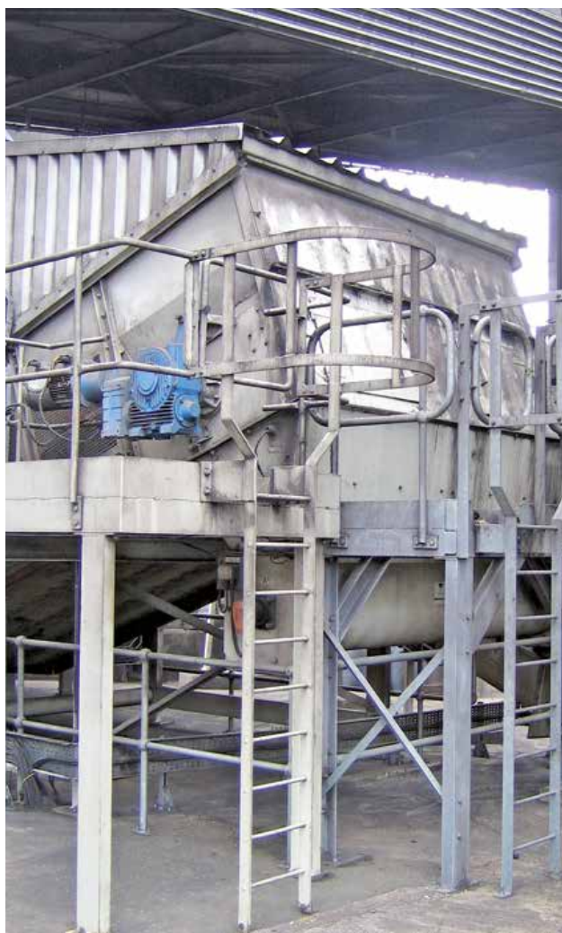
Transfer by Screw Feeder and Conveyor
