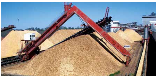
Longitudinal Storage with Portal Reclaimer by SCHADE
