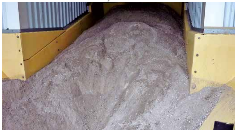
Samson® Material Feeder raised discharge permits transfer direct to surface mounted belt conveyor
