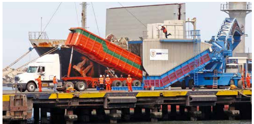
Samson® Material Feeder integrated to a Mobile Shiploader receives copper and gold concentrate
