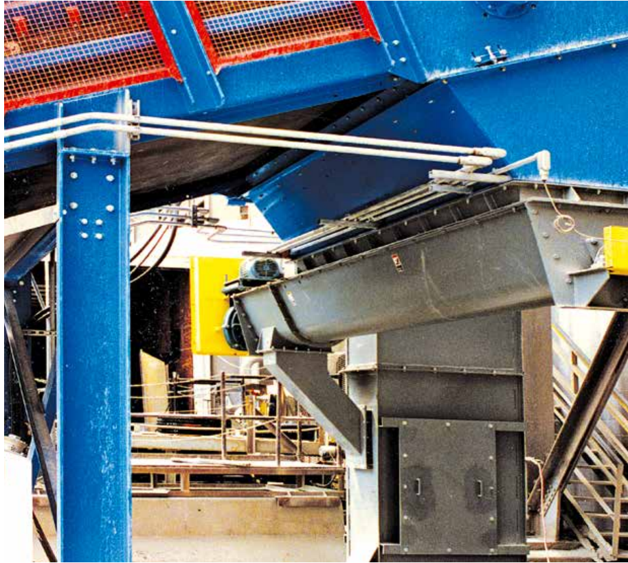
Single screw feeder provides metered output to a Bucket Elevator
