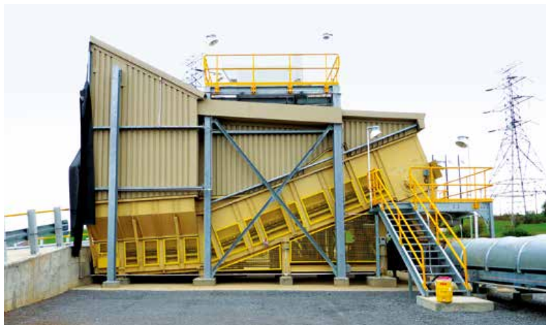
Samson® Material Feeder raised discharge permits transfer direct to surface mounted belt conveyor
