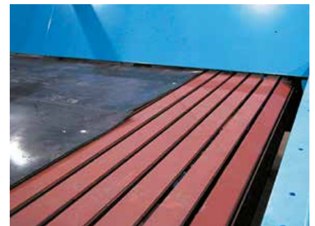
Steel apron bars support the load
