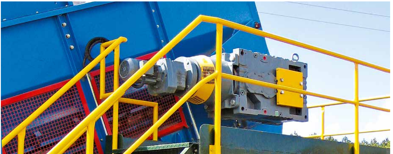
High efficiency helical/bevel main reduction gear with helical primary
