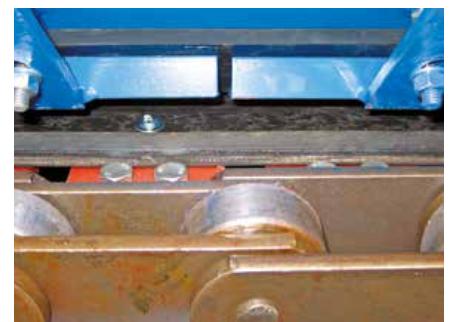
Load carried on the chain rollers
