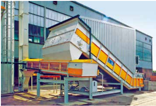
Kleen-line belt feeder transfer to Bucket Elevator
