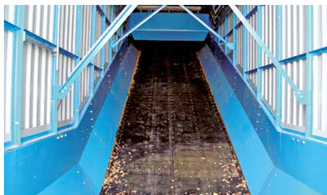
The wide apron-belt Samson® Material Feeder concept is ideal for difficult materials
