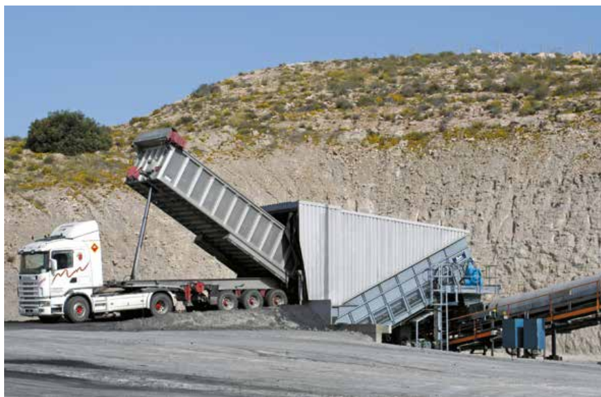
Samson® Material Feeder discharges direct to a surface mounted belt
