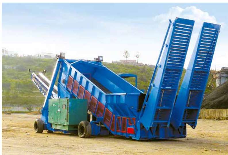
Stormajor® Boom Feeder supplied with powered travel and hinged truck ramps for easy manoeuvring around the stackyard
