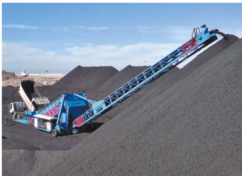
Stormajor® Boom Feeder supplied with powered travel and hinged truck ramps for easy manoeuvring around the stackyard
