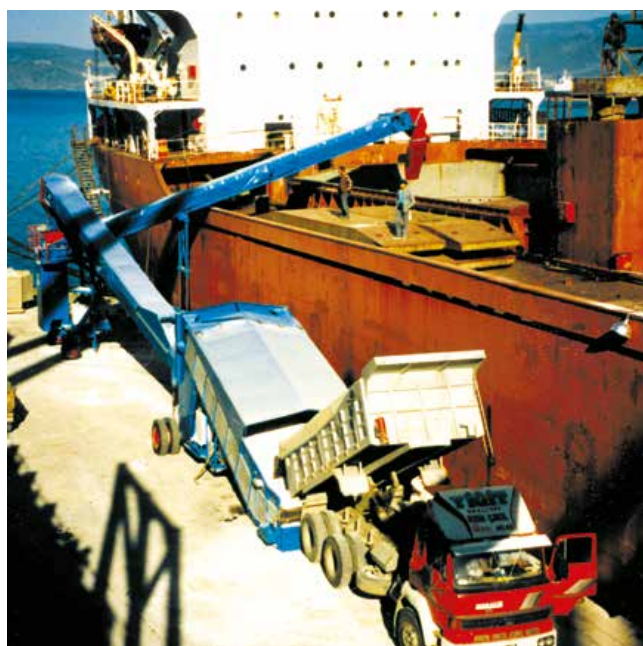
Shiploader + Stormajor® Boom Feeder for truck to ship loading
