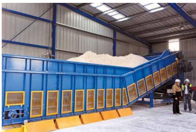
Samson® Material Feeder - Box Feeder for up to 120 tons live storage
