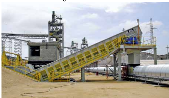
Samson® Material Feeder - Box Feeder for up to 120 tons live storage
