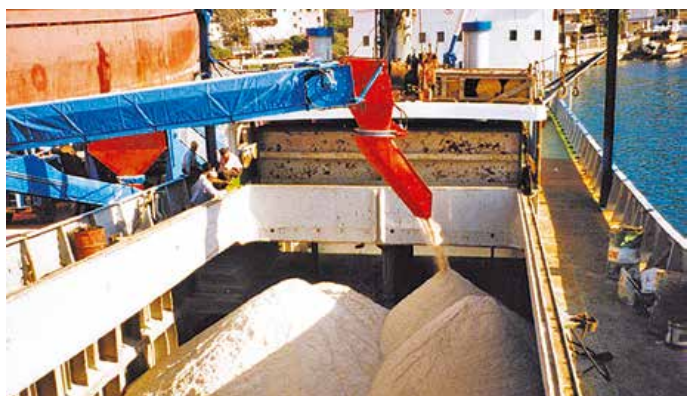
Trimming for small vessels using simple rotating chute
