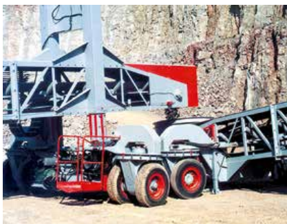
In-line or parallel travel for easy transfer point alignment
