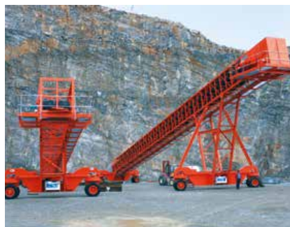
Two 50 metre x 1400 mm link conveyors
