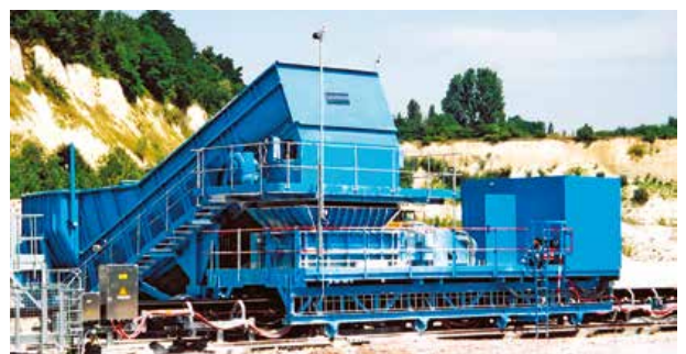
Overland Conveyor with Sledges for Lateral Movement Sizer with Drives and Controls mounted to Rail Bogie
