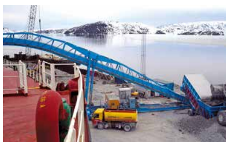
Cambered boom for maximum lift and outreach
