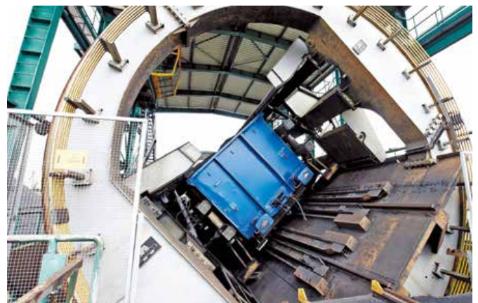
Wagon Tippler for Open Top Flat Bottom Wagons
