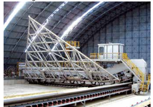
SCHADE bridge reclaimer for output homogenisation
