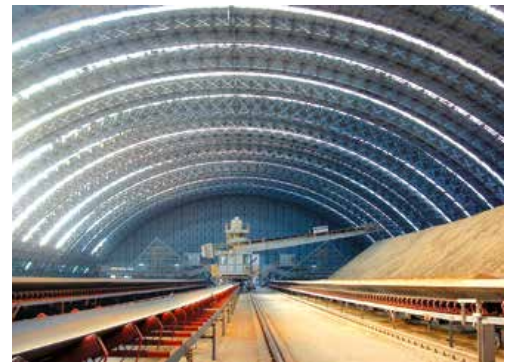
SCHADE blending bed storage with travelling stacker
