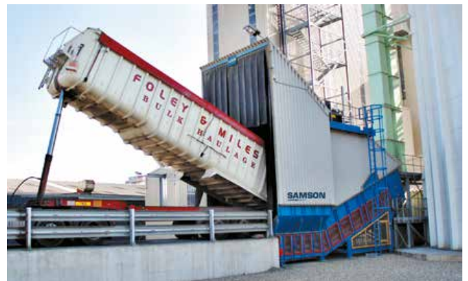
Samson® Material Feeder intake to process or batching plant
