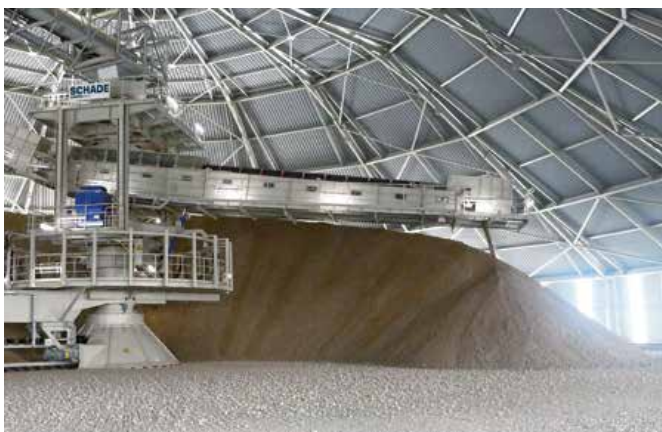
Circular Storage and Blending Bed by SCHADE
