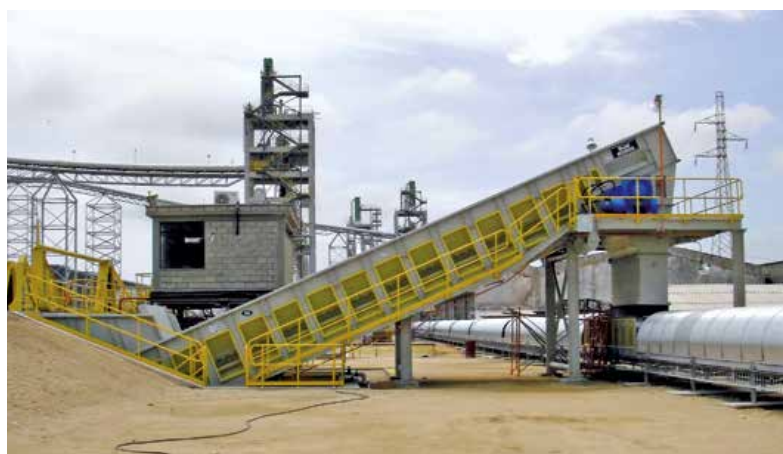
Samson® discharges directly to overland conveyor
