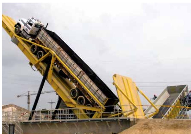
Hinged opening door combined with Tipping Platform
