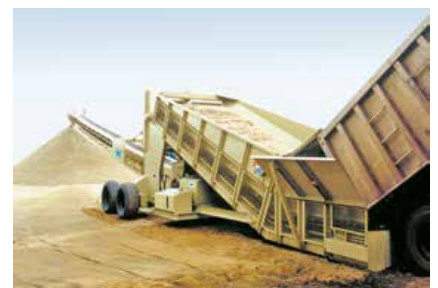
Direct receive from tipping or dump truck
