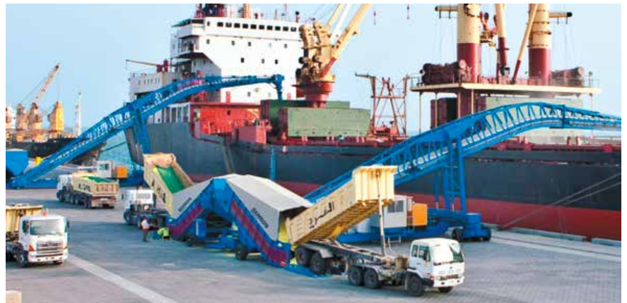
Twin Independent Samson® units feed a single Shiploader
