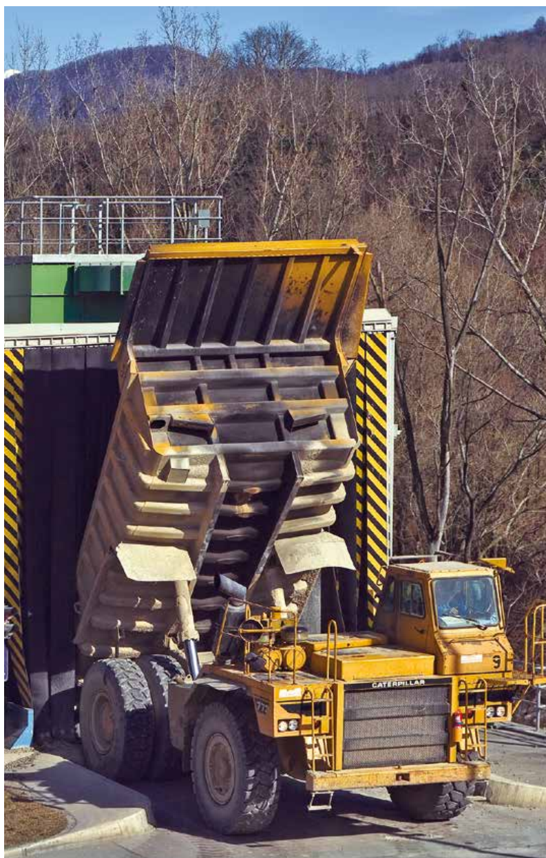
Intake direct from Haul Truck to Samson® Material Feeder
