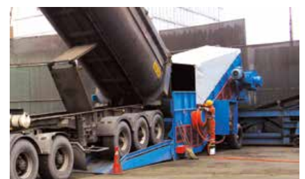
Independent Samson® feeds an existing shiploader
