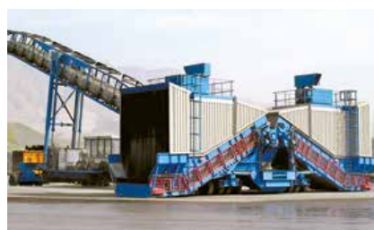
Simultaneous intake from two trucks
