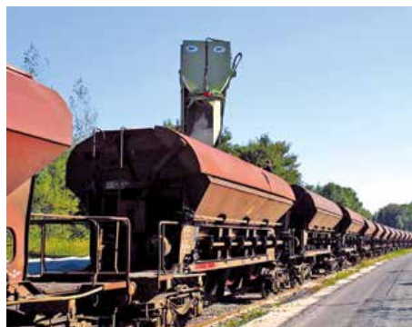
Rotating loading chute for accurate material placement
