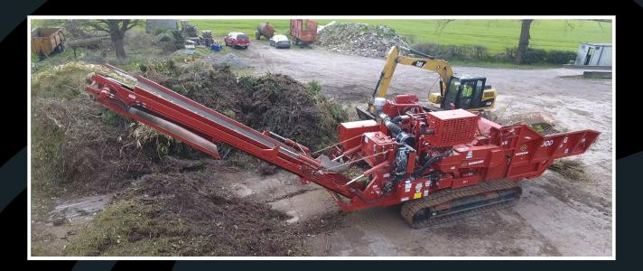
The Morbark 3200 Wood Hog is a horizontal shredder, aimed at wood and green waste applications, with logs up to a diameter of 36cm being shredded with ease. The unit comes on crawler tracks, allowing easy manoeuvrability around site. Its drive line protection system protects against major damage from contaminants.
