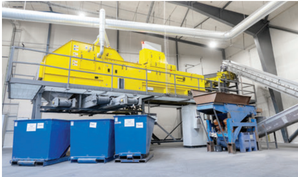
The upgrade to 11 t/h throughput makes the STEINERT PLASMAX | LIBS an absolute benchmark for sorting aluminium alloys. Photo: STEINERT
