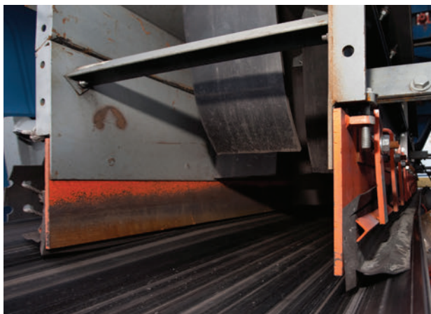
A properly structured enclosure is slightly elevated, with dust curtains, an external wearliner, and adequate skirting.
