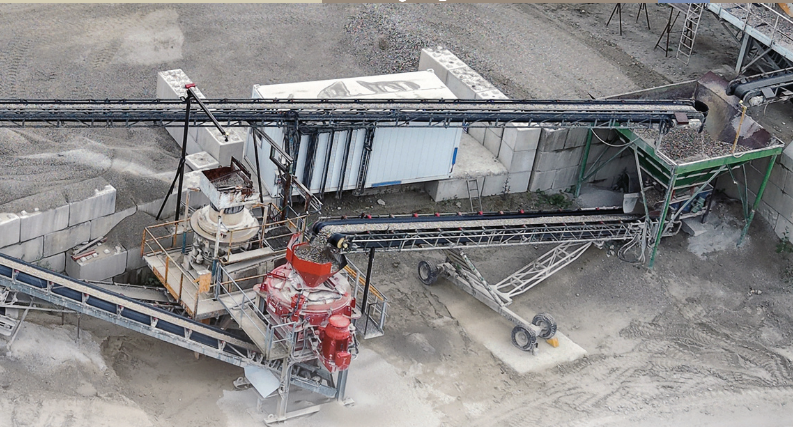
Moosleitner integrated the SBM V8 vertical impact crusher into his existing crushing plant.
