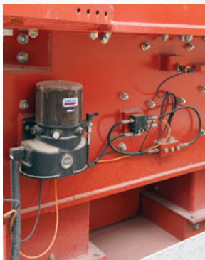
An automatic lubrication system minimises maintenance works at the SBM vertical impact crusher V8.
