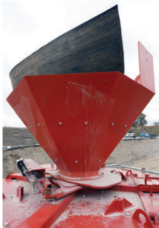
The patented SBM inlet control tightly closes the crushing chamber of the V8 vertical impact crusher, ensuring a stable material bed and low-dust operation of the crusher.
