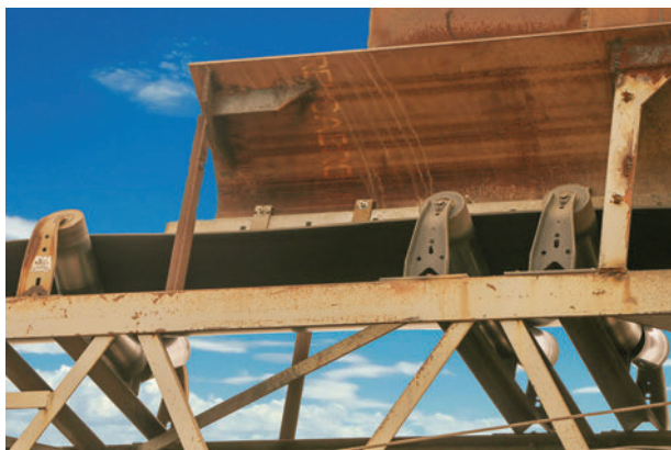
Figure 1 - This is an example of a fabricated curved skirtboard, which is hard to maintain when replacing wear liners and skirting.
